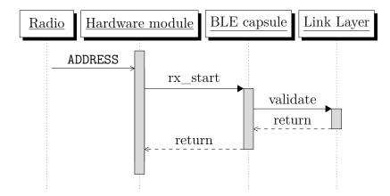
**Figure 5.2:** An ADDRESS event causes the radio to generate an interrupt. This in turn triggers the process of validating the received packet.
