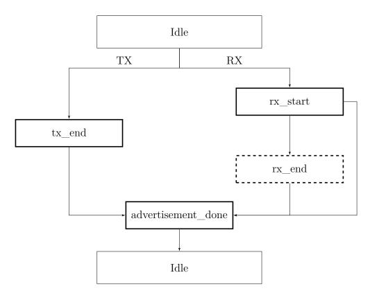
**Figure 4.2:** A flow chart showing the order of different events emitted by the hardware module.
