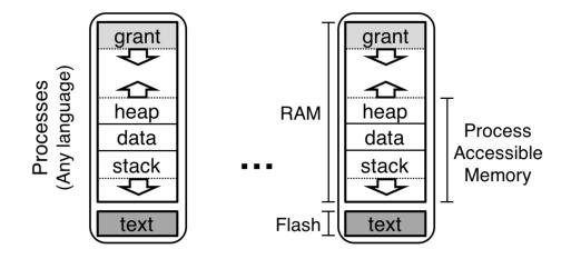
Figure 2.1: The memory of a process in Tock. Figure is from the paper "Multiprogramming a 64 kB Computer Safely and Efficiently" [1].
