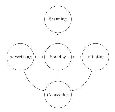
**Figure 2.2:** Bluetooth Low Energy Link Layer state machine and all the permitted transitions.
