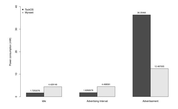
**Figure 6.5:** Bar chart comparing power consumption of Apache Mynewt and TockOS during different events in advertising.
