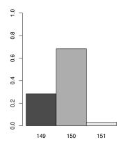
**Figure 6.7:** Bar chart comparing the ratio of packets received across the response time for the packet. Extreme values are not included in the figure.
