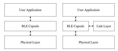
**Figure 4.1:** Comparison of Tock BLE stack before (left) and after (right) our design was implemented.
