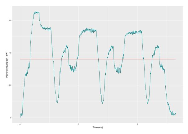
**Figure 6.4:** Graph showing Tock's power consumption during its active time period of an advertising event. The higher peaks (the first, third and fifth) represents when the radio is in TX mode, while the lower peaks (the second, fourth and sixth) is times when the radio is in RX mode. The average value is highlighted in orange.
