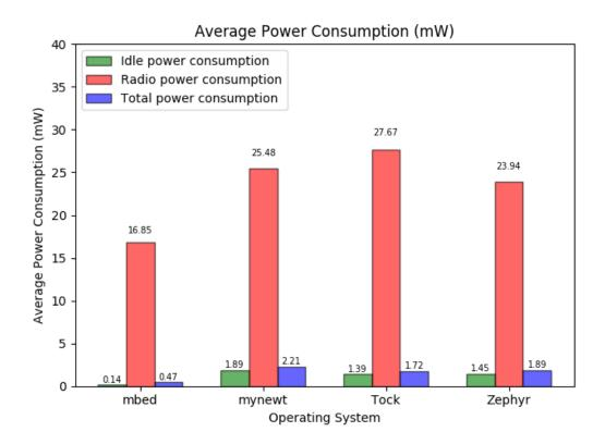
Figure 6.2: Embedded OS comparison BLE average power consumption. The y-axis shows the average power consumption in mW and the x-axis shows three different metrics of the average power consumption per operating system during BLE advertisements. The red bar shows the total average power consumption, the blue bar shows the average power consumption during the active time of the radio, and the green bar shows the average power consumption only during idle mode.
