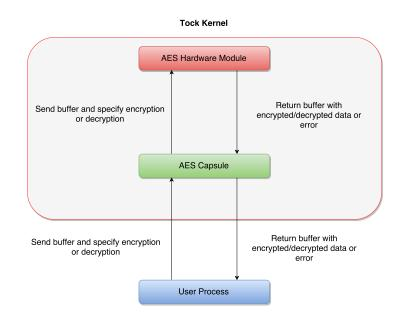
Figure 4.6: Tock AES device driver design. The figure illustrates the design of the device driver for the AES128 counter mode device driver. Green indicates that the module is safe, i.e., will not crash, whereas red contains unsafe code. Red modules rely on the fact that the programmers know what they are doing i.e., some of Rust safety features are disabled.
