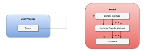
Figure 4.2: Device driver design hybrid. All or most of the device driver complexity is placed in the kernel, in the red box to the right. The user space application in the blue box to the left only invokes a function and the kernel handles the rest. However, this might increase the code size of the kernel but increase the performance. Further, the multiple arrows in the kernel indicate that a system call can utilize multiple kernel resources.
