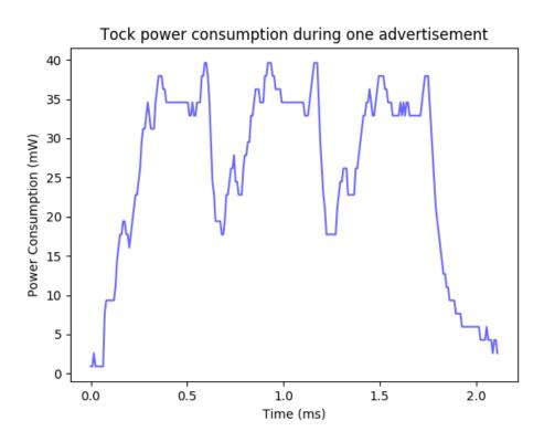
Figure 6.1: Tock power consumption during one advertisement. The figure shows the characteristics for the power consumption for one advertisement. During transmission, the power consumption increases which the spikes symbolize. The three spikes show the transmissions on the three advertisement channels. The y-axis shows the power consumption in mW and the x-axis shows the time in milliseconds.
