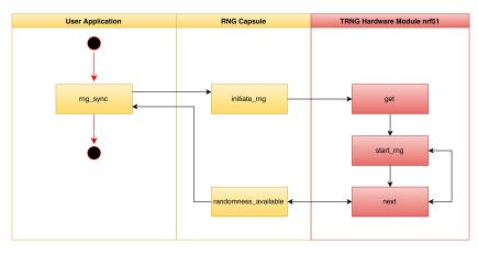
Figure 5.3: Tock TRNG device driver implementation. The figure shows the entire TRNG device driver. To the left and in the middle, yellow boxes are existing parts of Tock i.e., not implemented by us. To the right, red boxes are modules that directly configures the TRNG chip for nRF51 which have been implemented a part of this thesis.
