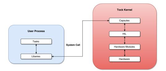
Figure 4.4: Tock device driver architecture. The blue box to the left represents the architecture for the user space application which contains two parts 1) the actual state machine 2) the libraries that provide a uniform usage of the device drivers and standard C functions. Furthermore, the red box to the right is the kernel architecture of the device drivers whereas capsules and hardware modules interact via a dedicated interface, HIL, to utilize hardware resources.
