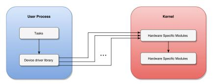
Figure 4.1: Device driver design micro. Favor flexibility to the developer whereas the majority of the complexity is maintained by the device driver library in user space, located in the blue box to left. In order to interact with the hardware, a system call needs to be performed. Thus, the kernel in the red box to the right does only manage basic hardware operations and introduce a system calls for every specific task which the arrows indicate.
