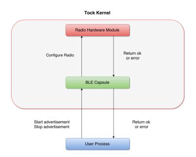
Figure 4.5: Tock BLE device driver design. The figure illustrates the design of the device driver for the BLE device driver. Green indicates that the module is safe, i.e., will not crash, whereas red contains unsafe code. Red modules rely on the fact that the programmers know what they are doing i.e., some of Rust safety features are disabled.
