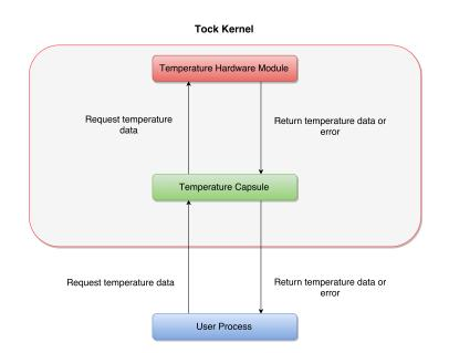
Figure 4.8: Tock temperature sensor device driver design. The figure illustrates the design of the device driver for the temperature sensor device driver. Green indicates that the module is safe, i.e., will not crash, whereas red contains unsafe code. Red modules rely on the fact that the programmers know what they are doing i.e., some of Rust safety features are disabled.
