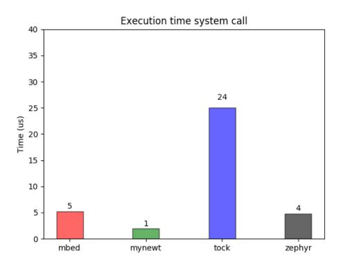
Figure 6.4: Embedded OS comparison average execution time of a system call. The y-axis is the execution time for one system call in  $\mu$ s and the x-axis is one for each of the operating systems. The results show that Mynewt is the fastest, mbed, and Zephyr are around 5 times slower and Tock is around 24 times slower. Tock stands out in this comparison and one reason is that the context switch assumes there exist an MPU which requires about 100 extra clock cycles.
