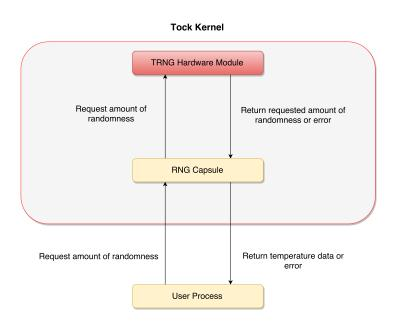
Figure 4.7: Tock TRNG device driver design. The figure illustrates the design of the device driver for the TRNG device driver. Green indicates that the module is safe, i.e., will not crash, whereas red contains unsafe code. Red modules rely on the fact that the programmers know what they are doing, i.e., some of Rust safety features are disabled.
