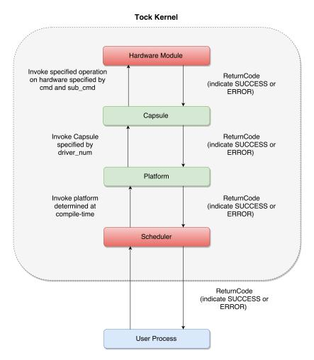
Figure 2.2: Tock system call. Showing the interaction flow upon a system call from a user space process to the Tock kernel. The blue box at the bottom is the user process outside the Tock kernel and the big gray box is the Tock kernel. Inside the Tock kernel, red boxes are the trusted modules and green boxes are the untrusted modules. The return code is returned to the user space process after the Tock kernel has handled the system call and it is either a success or an error code.
