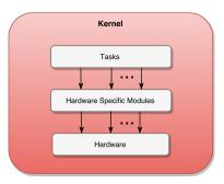
Figure 4.3: Device driver design monolithic. All functionality is integrated into a stripped variant of the kernel with the user space application as a part of the kernel. Unused kernel modules can be removed to provide lower memory footprint.
