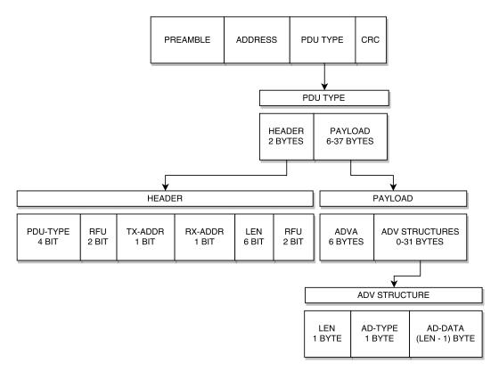
Figure 2.3: BLE advertisement packet structure. The figure illustrates a BLE packet specified by SIG. It describes the different layers from over the air structure to the different data structures to transmit in the BLE packet. The payload can consist of zero or several advertisement structures as long as it does not exceed 31 bytes.
